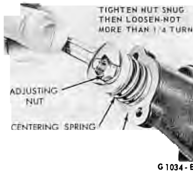
FIG. 17—Adjusting Centering Spring
