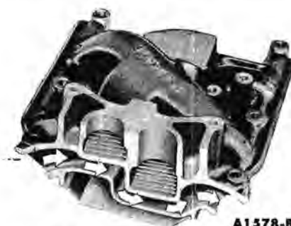
FIG. 5—Intake Manifold Exhaust Gas Crossover Passage
