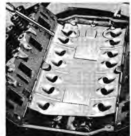
FIG. 62—Baffle Plate Removal
