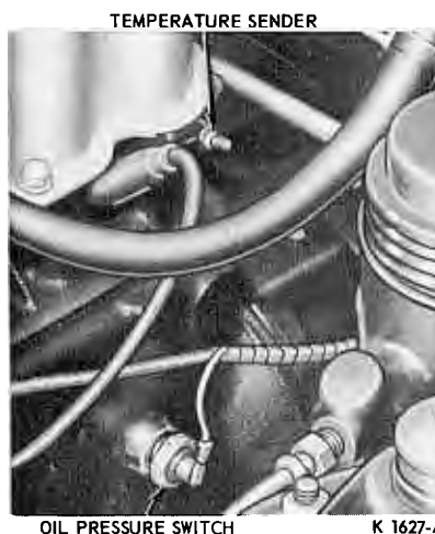
FIG. 3—Temperature and Oil Pressure Sender—Fairlane 6
