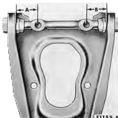
FIG. 6—Shaft Centered in Arm—Typical
