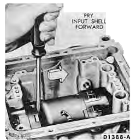
FIG. 38—Removing Front Pump
