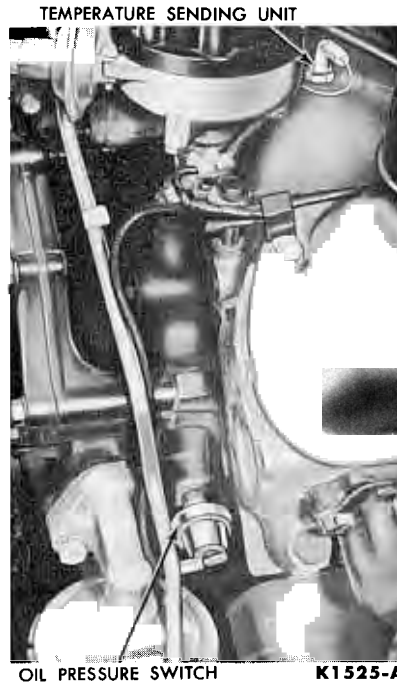
FIG. 2—Temperature Sender and Oil Pressure Switch—Falcon and Comet V-8
