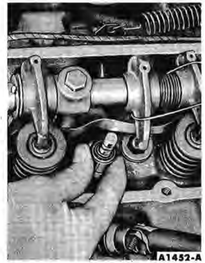
FIG. 24—Valve Stem Seal Removal
