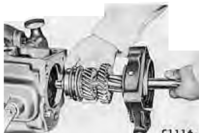
FIG. 13—Removing Output Shaft and Adapter
