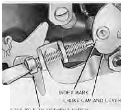
FIG. 10—Manual Choke Fast (Cold Engine) Idle Speed Adjustment
