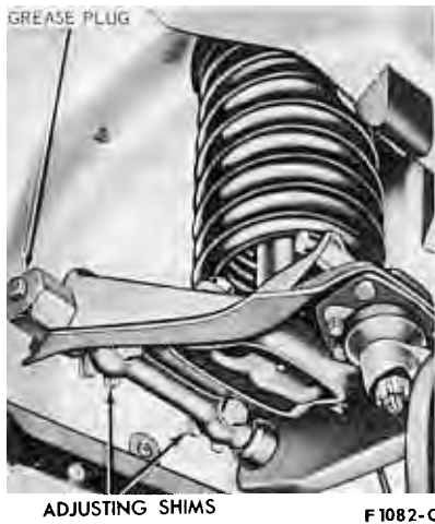
FIG. 7—Caster and Camber Adjustments—Mustang
