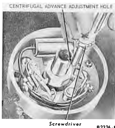
FIG. 18—Dual Point Distributor Centrifugal Advance Adjustment
