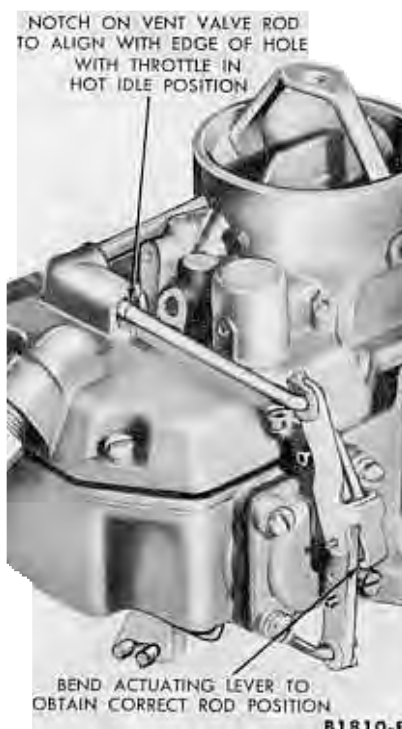
FIG. 24—Vent Valve Adjustment
