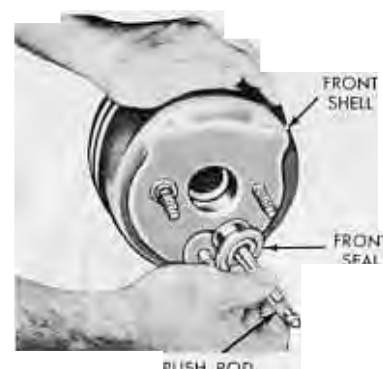
FIG. 36—Removing Front Seal and Push Rod—Bendix Booster
