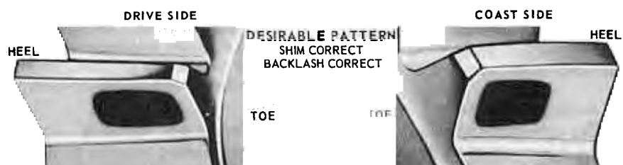
FIG. 2—Ideal Tooth Pattern—Integral Carrier Type Axle
