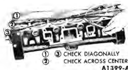
FIG. 29—Typical Cylinder Head Flatness
