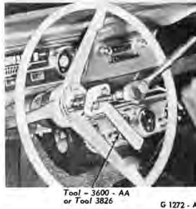
FIG. 5—Removing Steering Wheel—Typical
