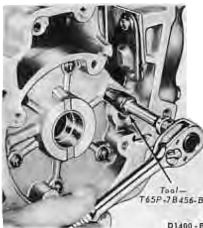
FIG. 50—Removing One-Way Clutch Outer Race Attaching Bolts
