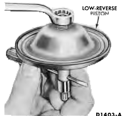
FIG. 52—Removing or Installing Low-Reverse Servo Piston
