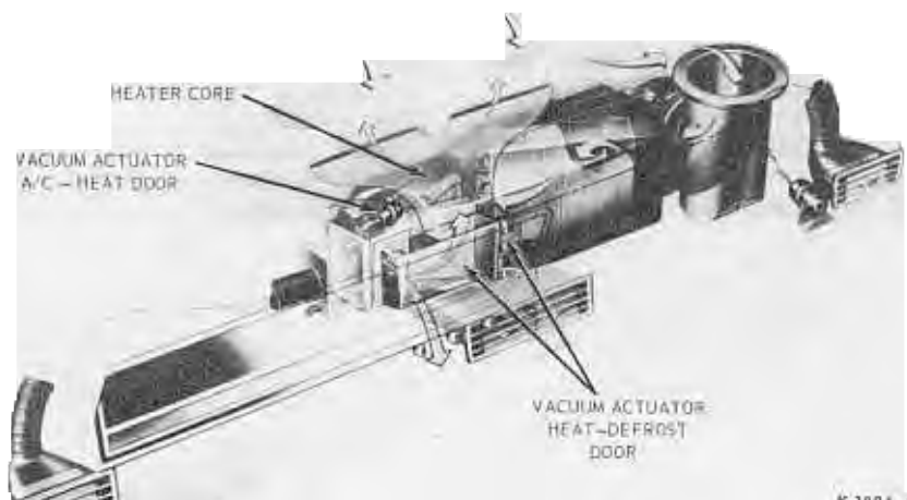
FIG. 2—Comet, Falcon and Fairlane A/C-Heater Air Flow—HEAT
