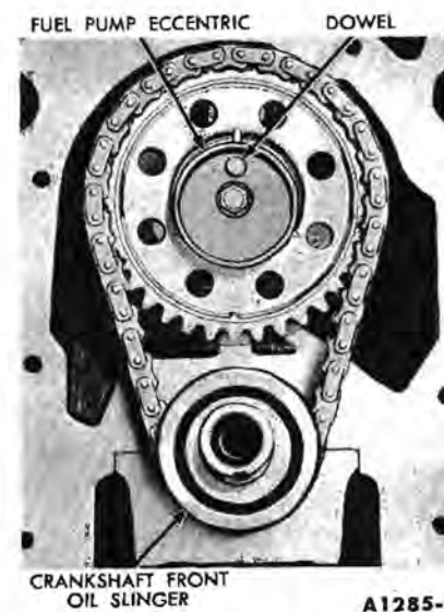
FIG. 32—Fuel Pump Eccentric and Front Oil Slinger Installed
