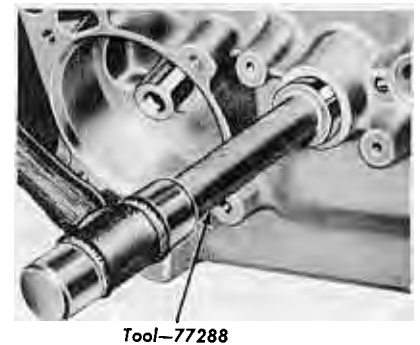
FIG. 61—Installing Manual Lever Seal
