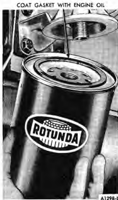
FIG. 51—Rotunda Oil Filter Replacement
