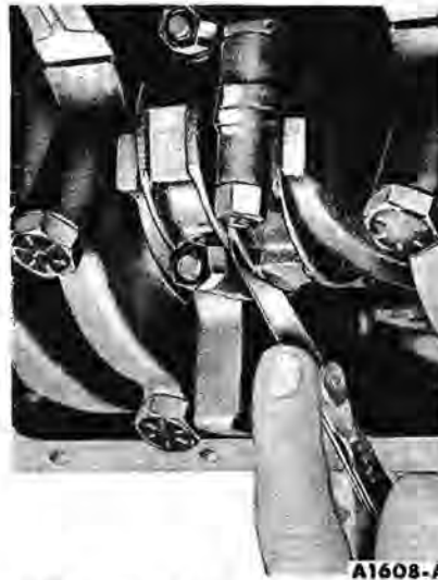
FIG. 45—Connecting Rod Side Clearance
