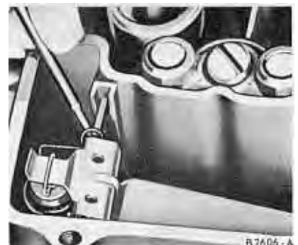
FIG. 13—Float Shaft Retainer Removal or Installation MAIN BODY
