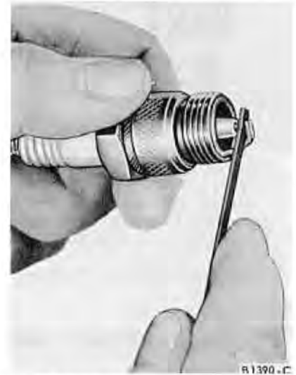
FIG. 31—Cleaning Spark Plug Electrode
