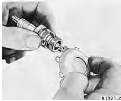
FIG. 21—Gapping Spark Plug
