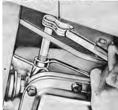
FIG. 22—Low-Reverse Band Adjustment
