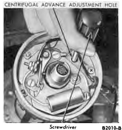
FIG. 16—Centrifugal Advance Adjustment
