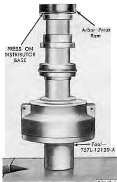
FIG. 12—Upper Bushing Installation
