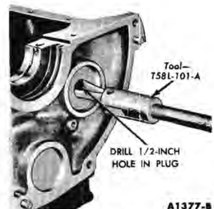
FIG. 33—Camshaft Rear Bearing Bore Plug Removal
