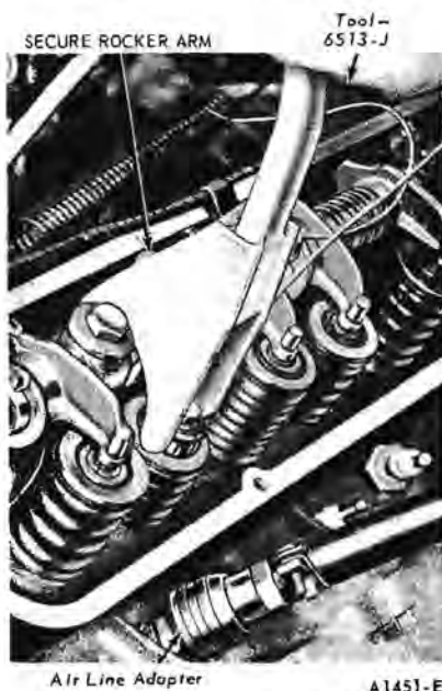
FIG. 26—Compressing Valve Spring—In Chassis
