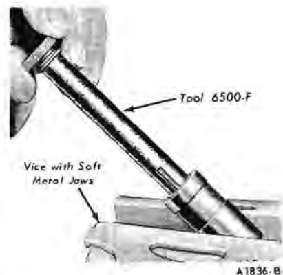
FIG. 36—Lifter Plunger Removal
