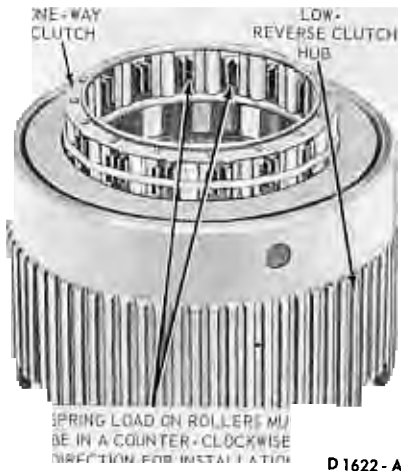
FIG. 59—Installing One-Way Clutch
