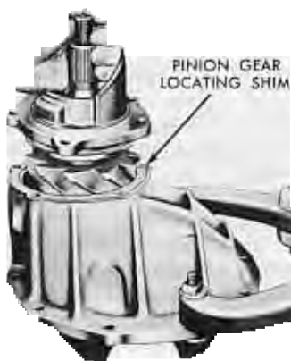
FIG. 48—Installing Pinion and Retainer
