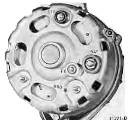
FIG. 7—Alternator Terminal Locations
