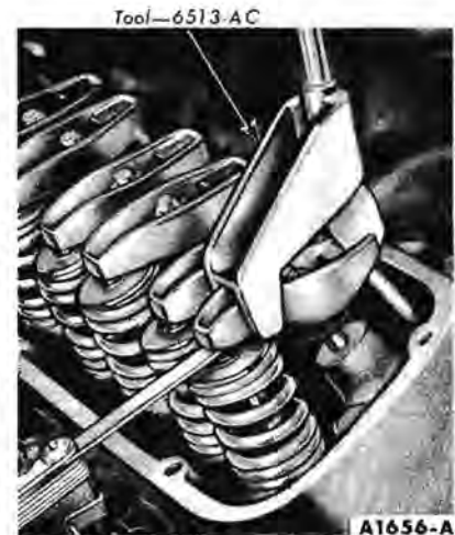
FIG. 16—Typical Valve Clearance Check—289 V-8
