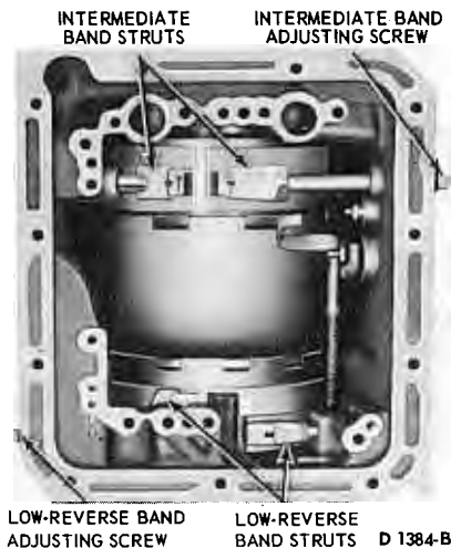
FIG. 34—Band Adjusting Studs and Struts
