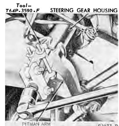
FIG. 7—Removing Pitman Arm—Typical
