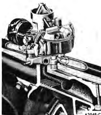
FIG. 5—Typical Coolant-Heated Carburetor Spacer
