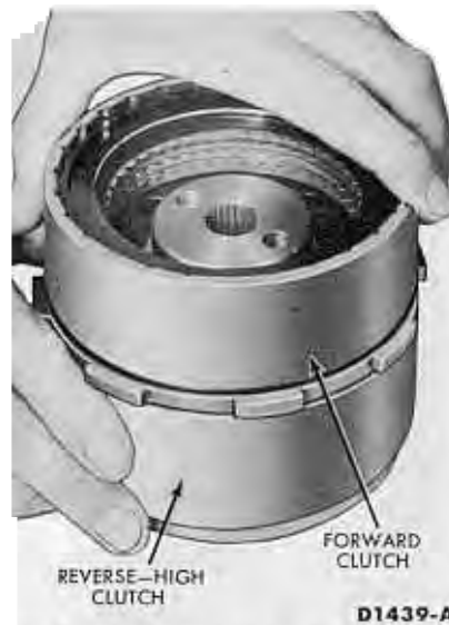
FIG. 96—Installing Clutch Units
