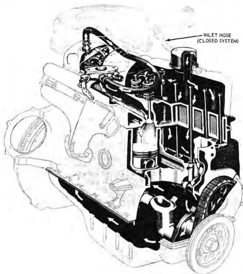
FIG. 8—Typical Positive Crankcase Ventilation System
