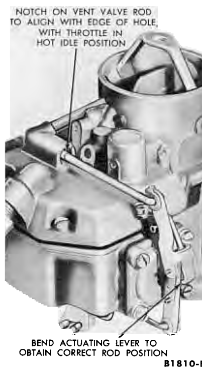
FIG. 14—Vent Valve Adjustment
