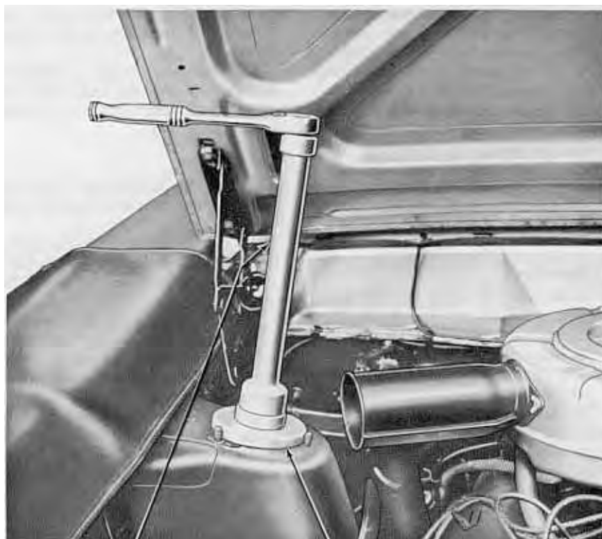
FIG. 12—Spring Compressor Installed—Upper View—Comet, Falcon and Fairlane
