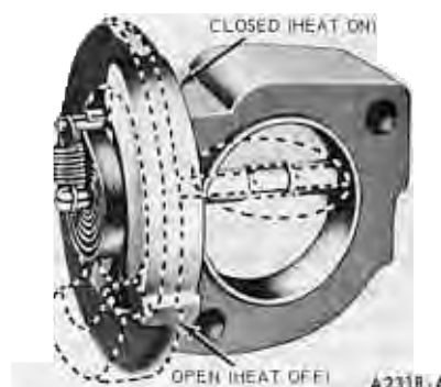
FIG. 1—390 V-8 Engine Exhaust Control Valve
