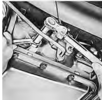
FIG. 21—Intermediate Band Adjustment
