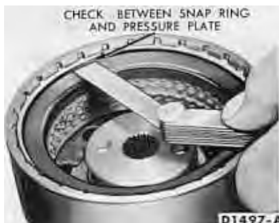
FIG. 80—Checking Forward Clutch Snap Ring Clearance
