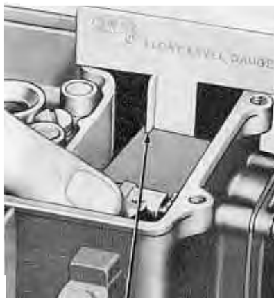
FIG. 5—Fuel Level Float Adjustment (Dry)—Ford 2-V and 4-V
