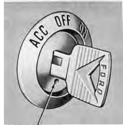
FIG. 6—Typical Ignition Switch Removal
