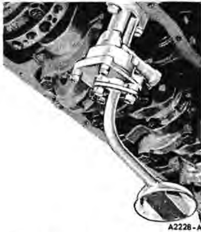
FIG. 47—200 Six Oil Pump Inlet Tube Installed
