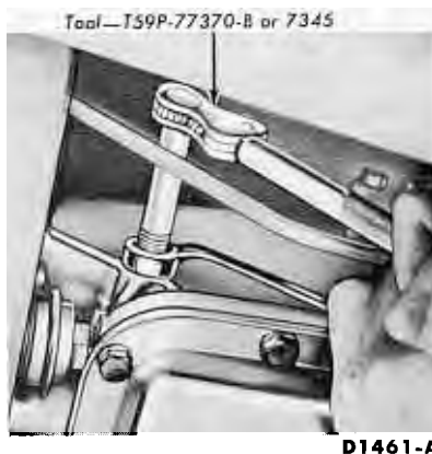
FIG. 25—Low-Reverse Band Adjustment
