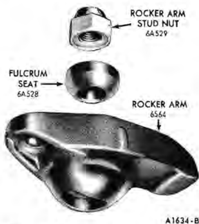
FIG. 18—Valve Rocker Arm Assembly
