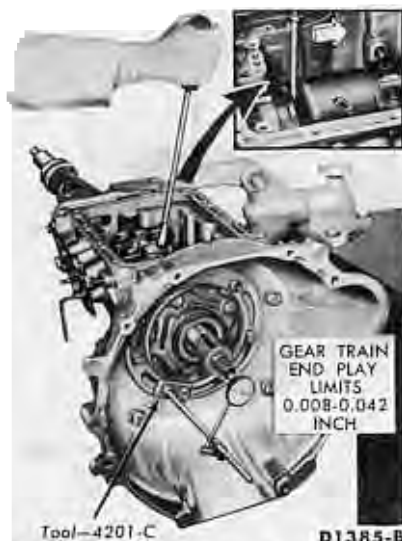
FIG. 35—Checking End Play
