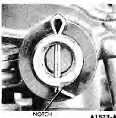
FIG. 14—Typical Installation Identification Mark—Rocker Arm Shaft Assembly
