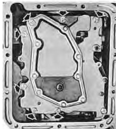
FIG. 33—Control Valve Attaching Bolts
