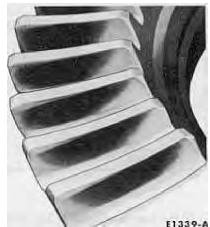
FIG. 6—Unacceptable Non-Hunting Pattern—Center-Heel-Center
