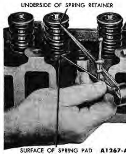
FIG. 22—Valve Spring Assembled Height
