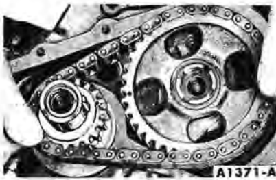
FIG. 27—Timing Chain and Sprockets Removal
