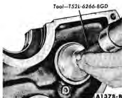
FIG. 34—Camshaft Rear Bearing Bore Plug Installation
