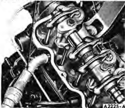
FIG. 24—Compressing Valve Spring—In Chassis
