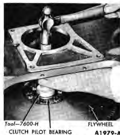
FIG. 49—Typical Clutch Pilot Service Bearing Installation
