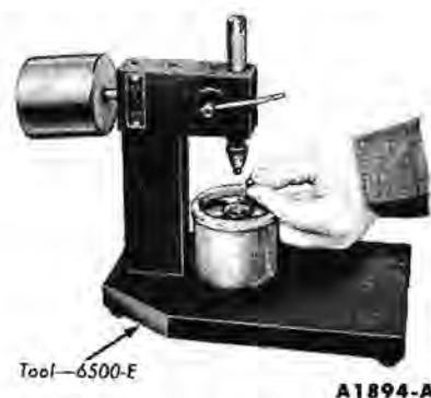
FIG. 4—Placing Steel Ball in Valve Lifter Plunger
