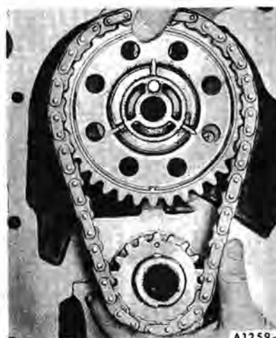
FIG. 30—Timing Chain Removal or Installation
