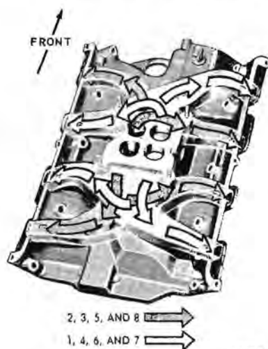
FIG. 4—Intake Manifold Fuel Passages
