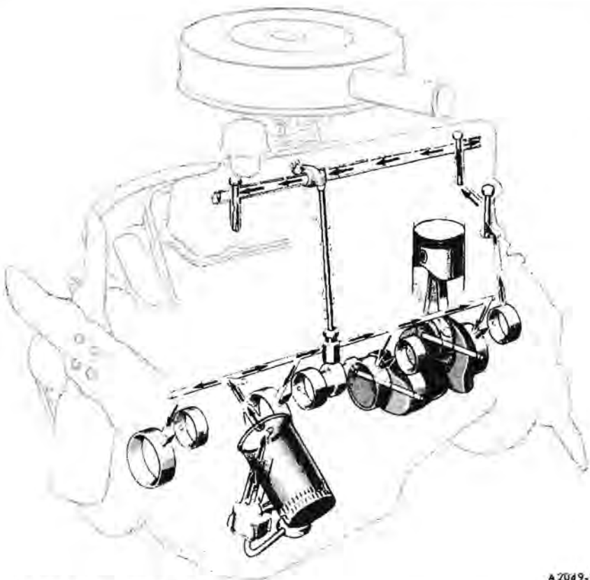
FIG. 7—Typical Lubrication System
