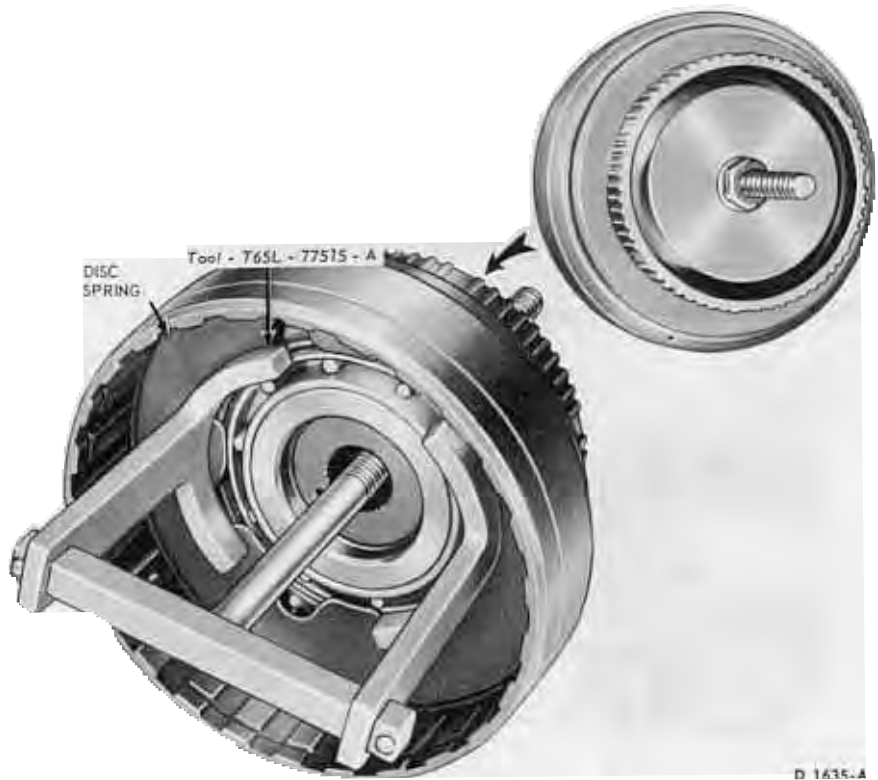
FIG. 52—Removing or Installing Disc Spring
