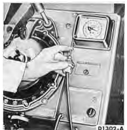
FIG. 7—Testing Transmission Vacuum Unit for Leakage
