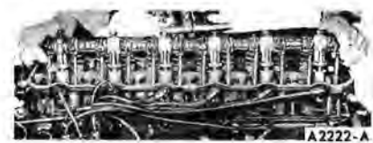
FIG. 16—Valve Rocker Arm Shaft Removal
