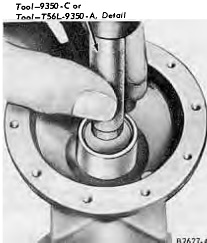
FIG. 6—Seating the Oil Seal
