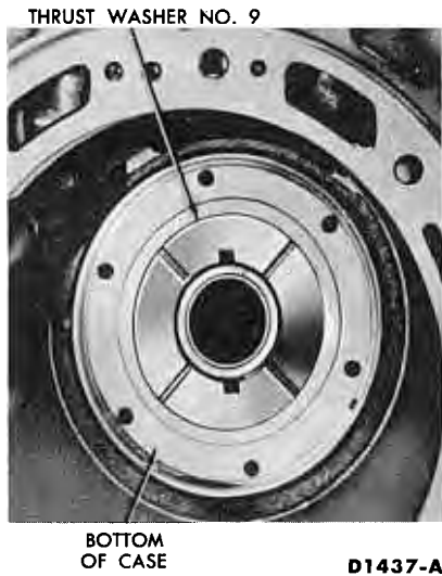
FIG. 88—Number 9 Thrust Washer Location
