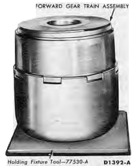
FIG. 42—Forward Part of Gear Train Positioned in Holding Fixture
