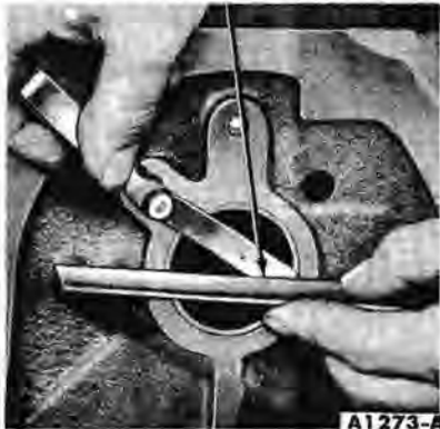
FIG. 60—Camshaft Front Bearing Measurement
