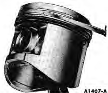
FIG. 27—Ring Side Clearance
