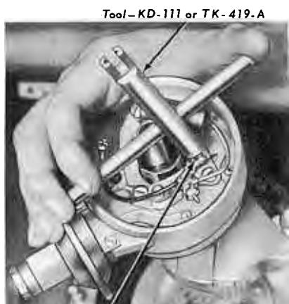
FIG. 20—Aligning Breaker Points
