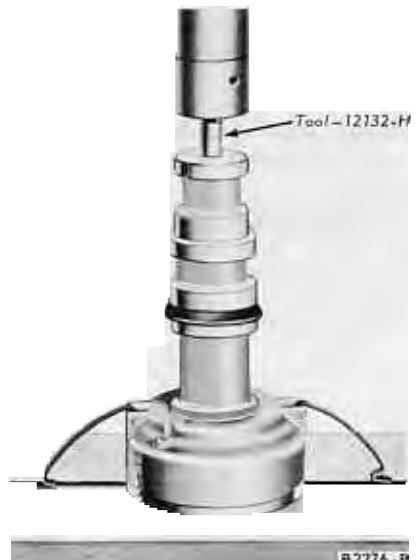
FIG. 11—Upper Bushing Removal
