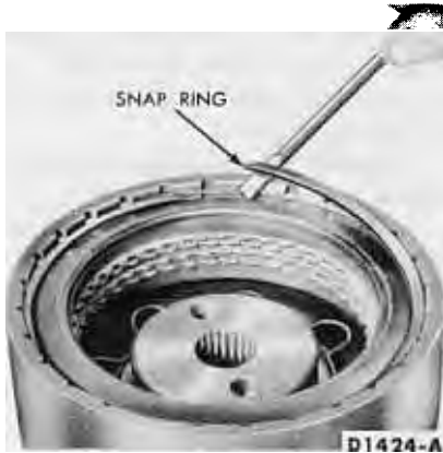
FIG. 50—Removing Forward Clutch Pressure Plate Snap Ring
