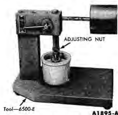
FIG. 5—Adjusting the Ram Length
