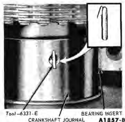
FIG. 39—Upper Main Bearing Insert Removal or Installation
