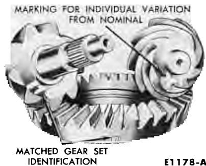
FIG. 44—Pinion and Ring Gear Markings
