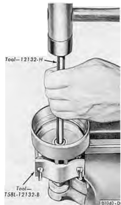
FIG. 9—Lower Bushing Removal
