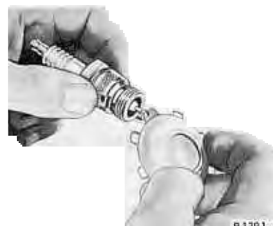
FIG. 28—Checking Spark Plug Gap
