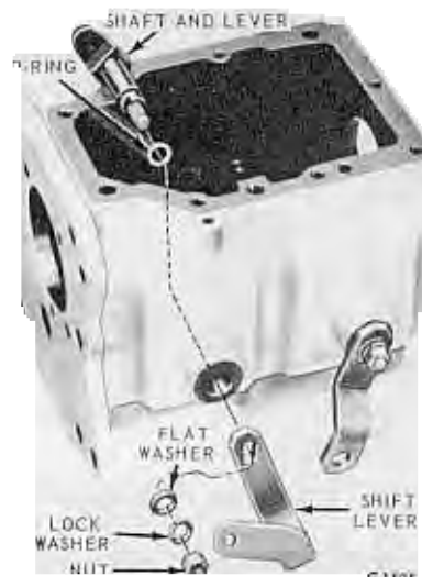
FIG. 14—Shift Lever and Shaft—Disassembled
