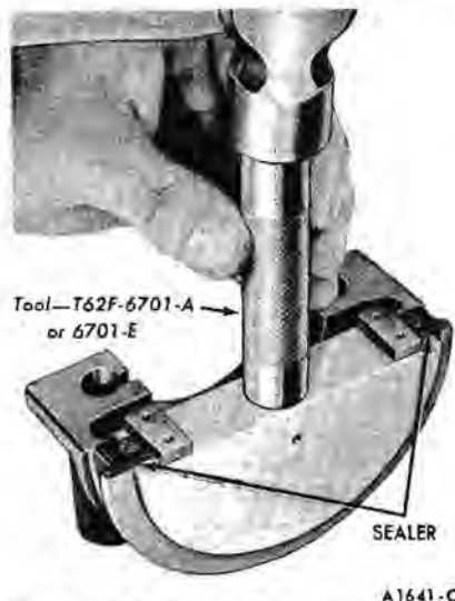
FIG. 42—Seal to Rear Bearing Cap Installation
