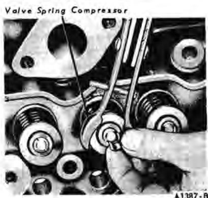
FIG. 21—Compressing Valve Spring—On Bench
