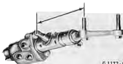
FIG. 8—Control Valve Length Adjustment—Mustang 6-Cylinder
