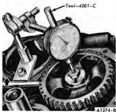
FIG. 11—Typical Camshaft End Play
