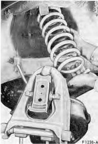
FIG. 10—Removing or Installing Spring—Mustang
