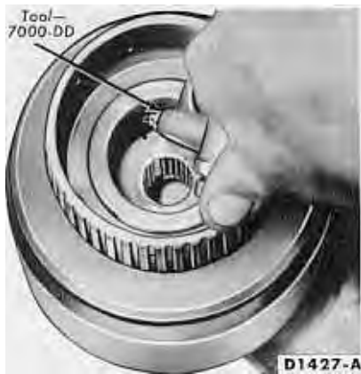
FIG. 53—Removing Forward Clutch Piston
