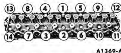
FIG. 20—Cylinder Head Bolt Torque Sequence
