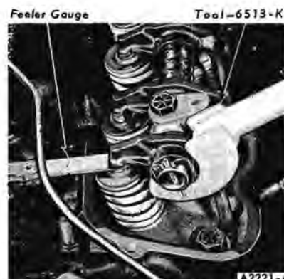
FIG. 13—Valve Clearance Check—170 and 200 Six
