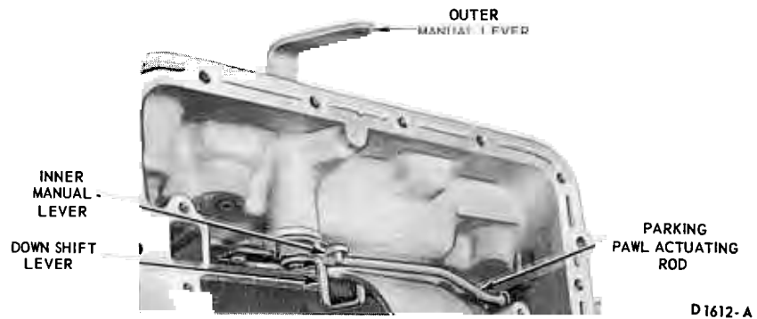
FIG. 32—Downshift and Manual Linkage
