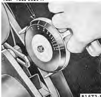
FIG. 18—Checking Drive Belt Tension
