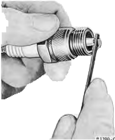
FIG. 20—Cleaning Plug Electrode
