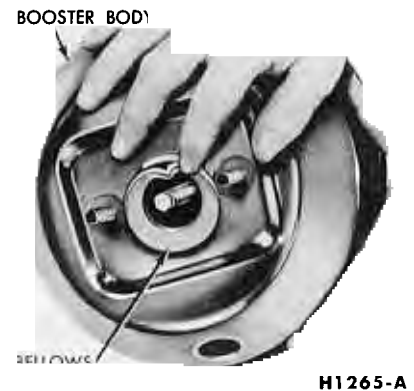
FIG. 43—Bellows to Booster Body Engagement—Midland-Ross
