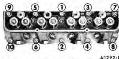
FIG. 19—Cylinder Head Bolt Torque Sequence
