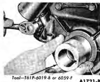
FIG. 36—Cylinder Front Cover Alignment
