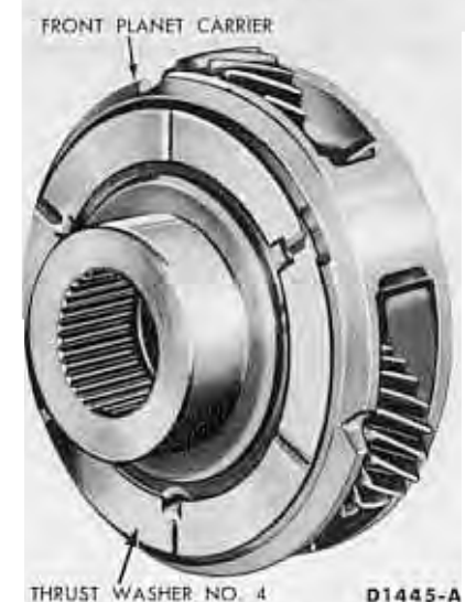
FIG. 99—Number 4 Thrust Washer Location
