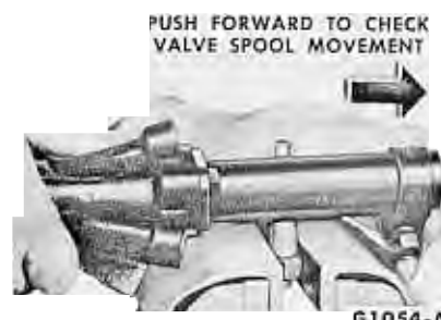
FIG. 18—Inspecting Valve Spool Movement
