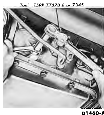
FIG. 23—Intermediate Band Adjustment
