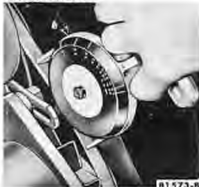
FIG. 2—Checking Drive Belt Tension
