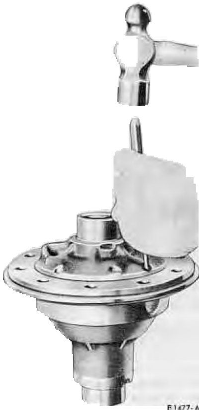
FIG. 20—Differential Pinion Shaft Lock Pin Removal
