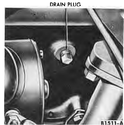
FIG. 22—Typical Cylinder Block Drain Plug
