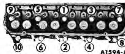
FIG. 25—Cylinder Head Bolt Torque Sequence
