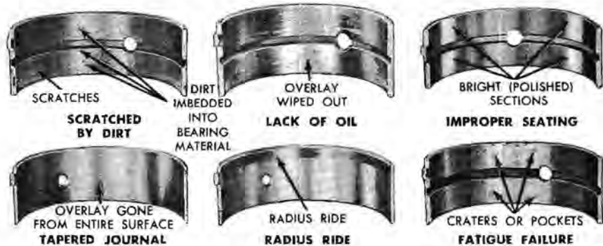
FIG. 39—Typical Bearing Failures
