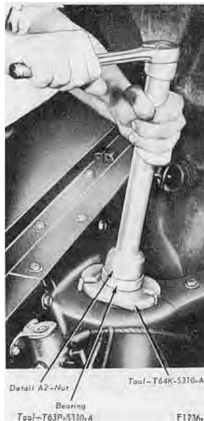
FIG. 8—Compressing or Releasing Spring on Mustang—Upper View
