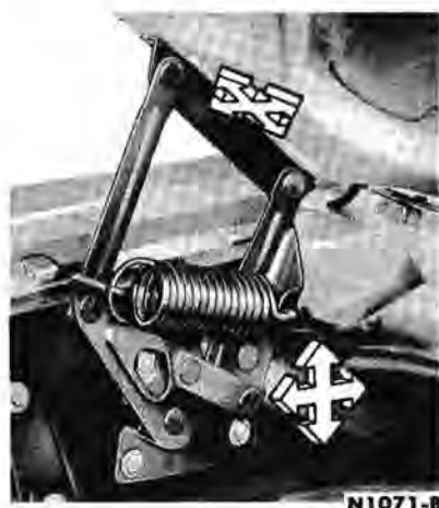
FIG. 1—Hood Hinge Installation—Typical
