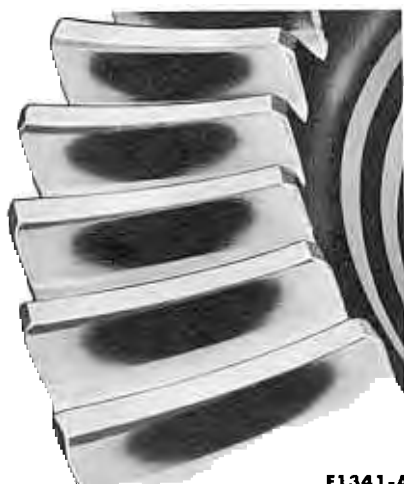
FIG. 8—Acceptable Non-Hunting Pattern—Uniform
