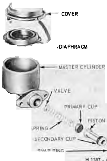
FIG. 33—Master Cylinder Used With Disc Brakes—Disassembled
