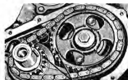
FIG. 26—Aligning Timing Marks
