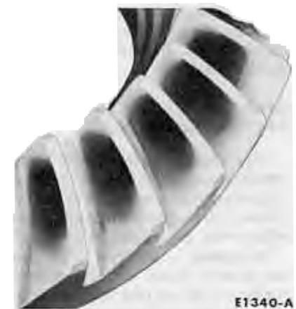
FIG. 7—Acceptable Non-Hunting Gear Set—Coast Pattern
