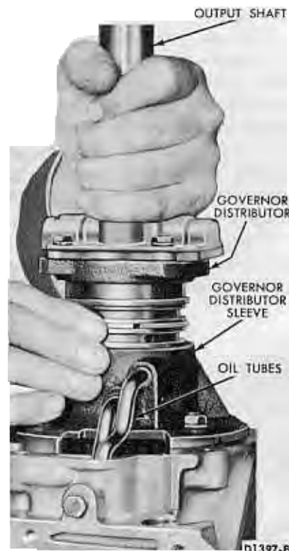
FIG. 47—Removing or Installing Output Shaft and Governor Distributor
