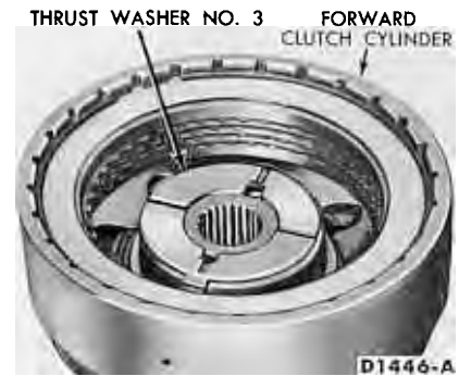
FIG. 97—Number 3 Thrust Washer Location
