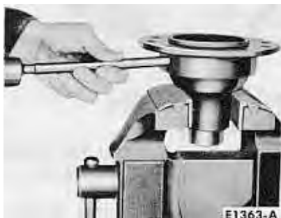
FIG. 33—Driving Out Differential Pinion Shaft
