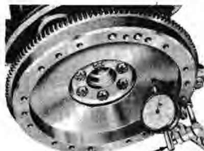
FIG. 9—Typical Flywheel Face Runout
