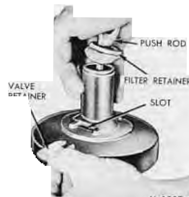
FIG. 39—Removing or Installing Valve Retainer—Bendix Booster
