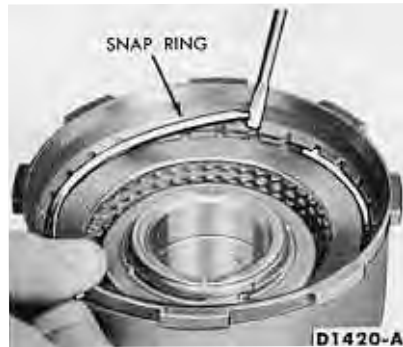
FIG. 45—Removing Reverse-High Pressure Plate Snap Ring
