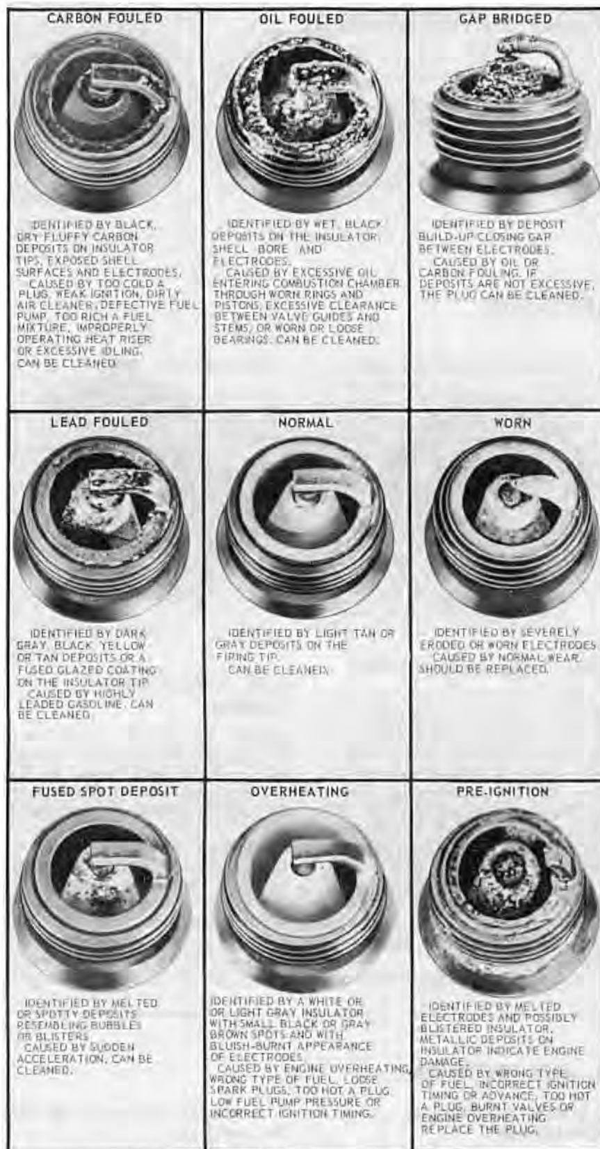
FIG. 30—Spark Plug Inspection
