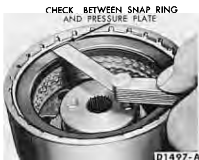
FIG. 54—Checking Forward Clutch Snap Ring Clearance
