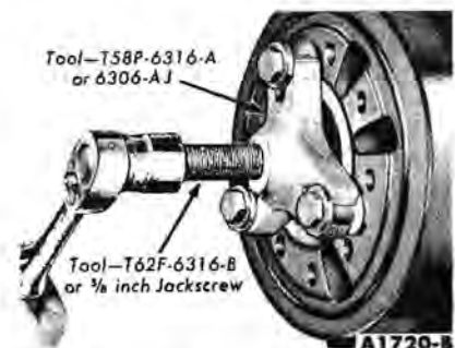
FIG. 31—Crankshaft Vibration Damper Removal
