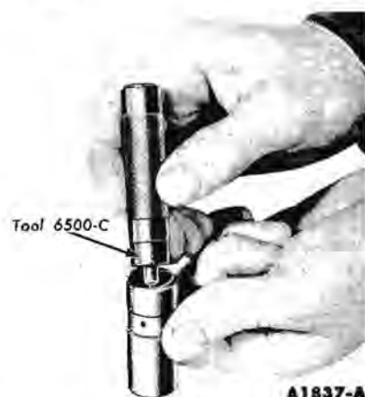
FIG. 38—Valve Lifter Lock Ring Installation
