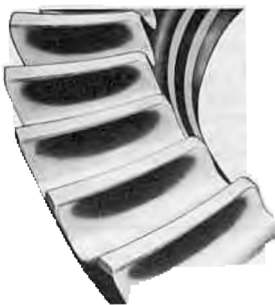
FIG. 3—Ideal Tooth Pattern—Removable Carrier Type Axle
