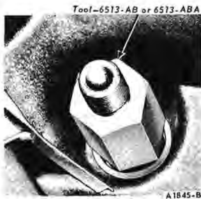
FIG. 25—Installation of Air Adapter Tool in Spark Plug Hole
