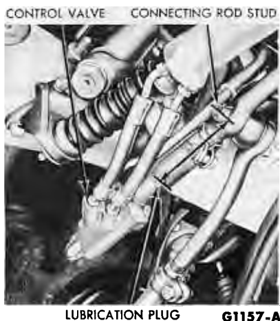
FIG. 10—Control Valve Installation Measurement—Typical—Comet, Falcon, and Fairlane
