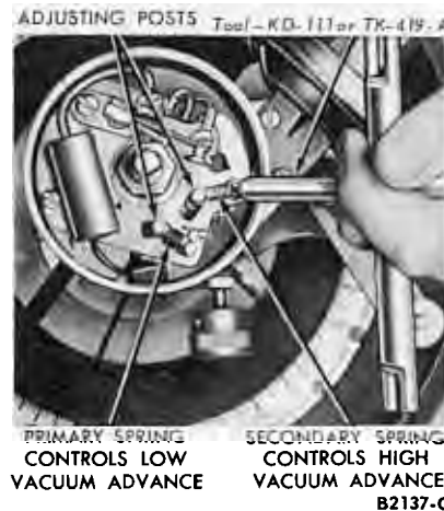
FIG. 15—Spark Advance Adjustment
