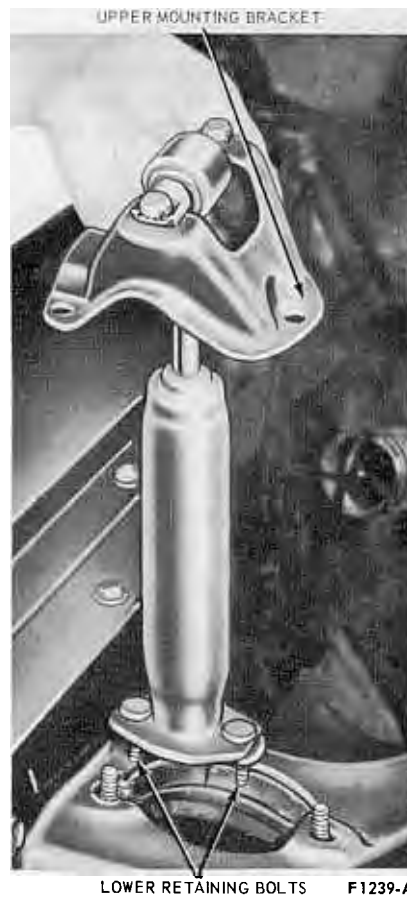
FIG. 15—Removing or Installing Front Shock Absorber—Typical
