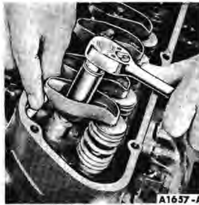
FIG. 15—Typical Valve Clearance Adjustment—289 V-8
