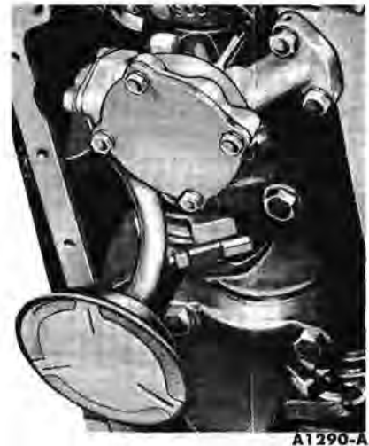
FIG. 52—Oil Pump and Inlet Tube Installed
