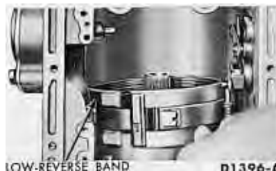
FIG. 46—Removing or Installing Low-Reverse Band
