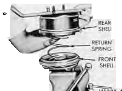
FIG. 37—Separating Booster Shells—Bendix Booster
