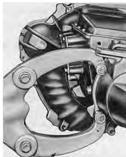
FIG. 32—Transmission Mounted in Holding Fixture
