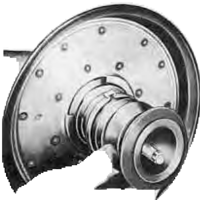
FIG. 44—Removing or Installing Rear Seal to End Plate—Midland-Ross
