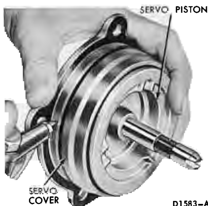
FIG. 54—Removing Intermediate Servo Piston—6 Cylinder Engine
