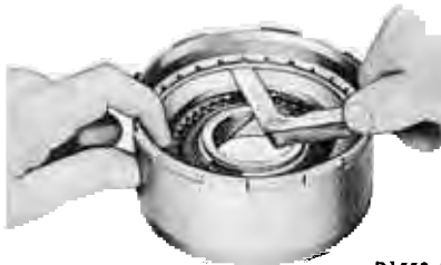
FIG. 49—Checking Reverse-High Clutch Snap Ring Clearance
