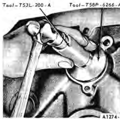
FIG. 61—Camshaft Rear Bearing Bore Plug Installation
