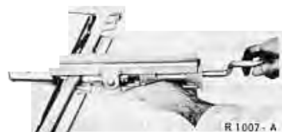
FIG. 15—Glass Channel Replacement
