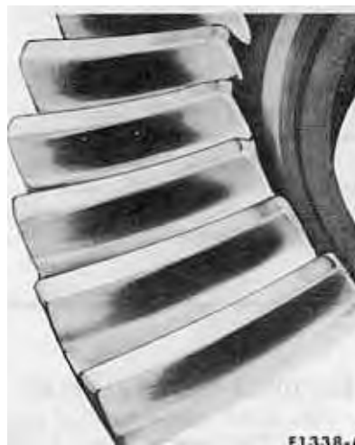
FIG. 5—Unacceptable Non-Hunting Pattern—Center-Toe-Center
