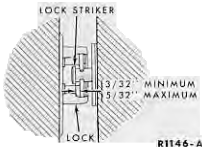
FIG. 1—Door Lock Striker Adjustment
