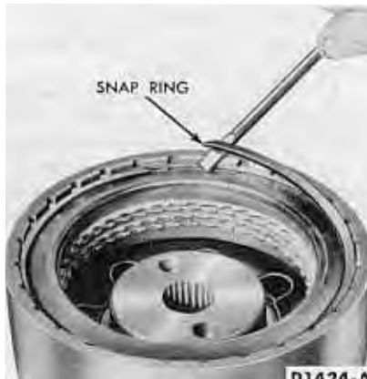
FIG. 76—Removing Forward Clutch Pressure Plate Snap Ring
