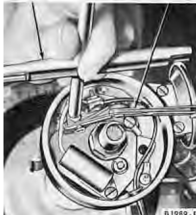
FIG. 21—Adjusting New Breaker Point Gap
