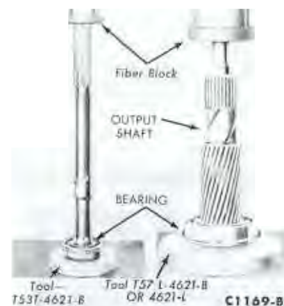
FIG. 11—Replacing Output Shaft Bearing
