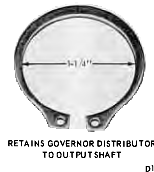
FIG. 92—Governor and Reverse Ring Gear and Hub Snap Ring Identification
