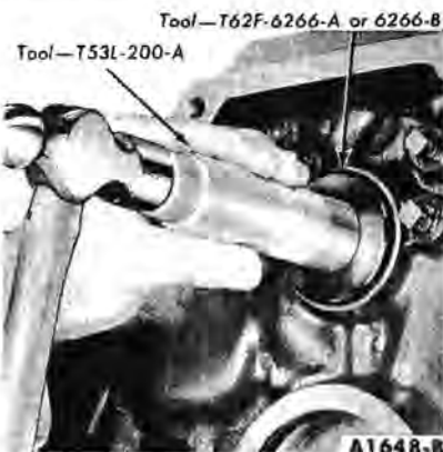
FIG. 63—Camshaft Rear Bearing Bore Plug Installation
