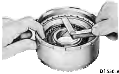
FIG. 75—Checking Reverse-High Clutch Snap Ring Clearance
