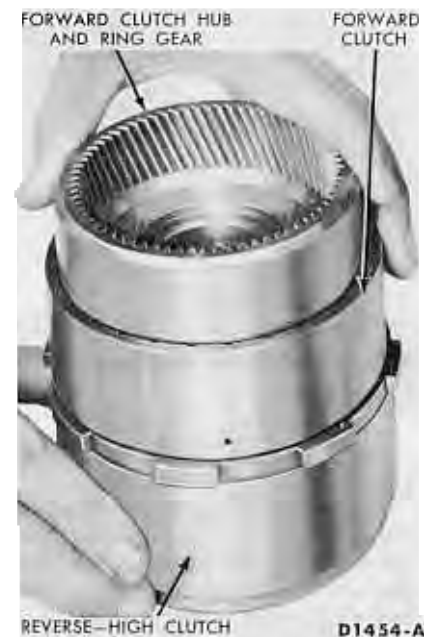
FIG. 98—Installing Forward Clutch Hub and Ring Gear
