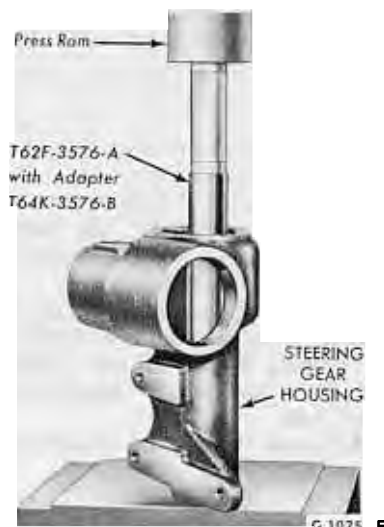
FIG. 11—Installing Sector Shaft Bearing
