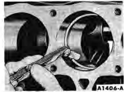
FIG. 26—Piston Ring Gap
