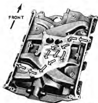
FIG. 3—Typical Intake Manifold Exhaust Gas Passages
