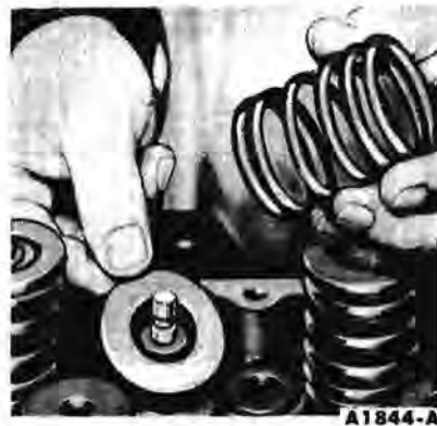
FIG. 23—Valve Spring Spacer Installation
