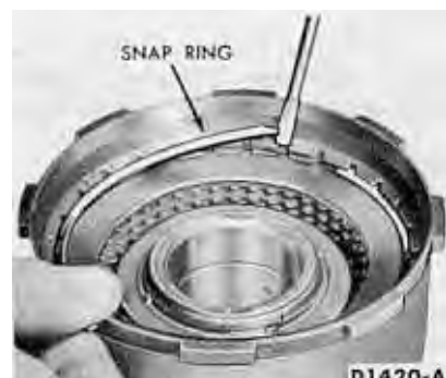
FIG. 71—Removing Reverse-High Clutch Snap Ring
