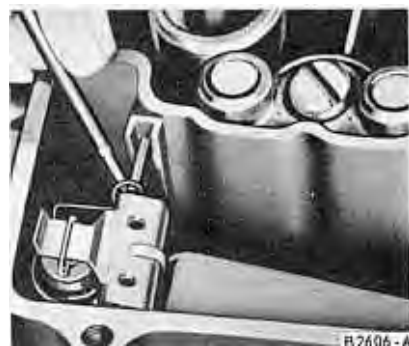
FIG. 18—Float Shaft Retainer Removal or Installation
