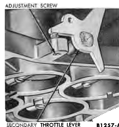
FIG. 6—Secondary Throttle Plate Adjustment—Ford 4-V
