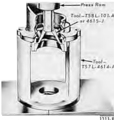
FIG. 42—Removing Pinion Bearing Cup
