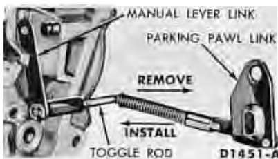
FIG. 58—Removing or Installing Parking Pawl Toggle Rod
