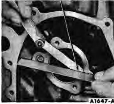
FIG. 62—Camshaft Front Bearing Measurement
