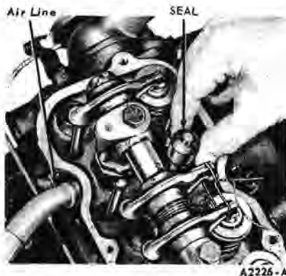
FIG. 25—Valve Stem Seal Removal
