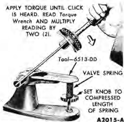
FIG. 34—Valve Spring Pressure
