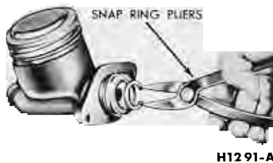
FIG. 32—Removing Snap Ring From Master Cylinder—Typical
