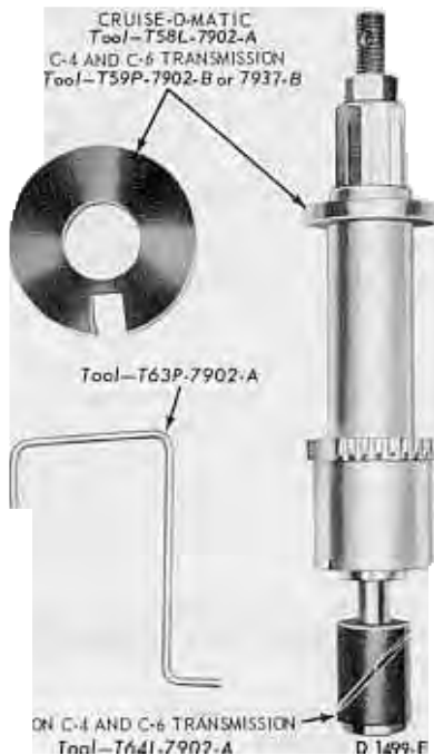
FIG. 10—Converter Checking Tool
